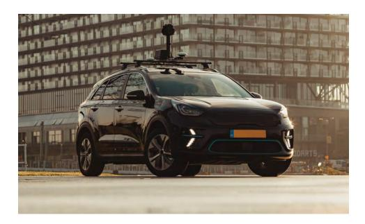
equipment to measure geographical information. The system measures the distance from the road to the vehicle and uses the new navigation data to improve their customers' mapping systems.
